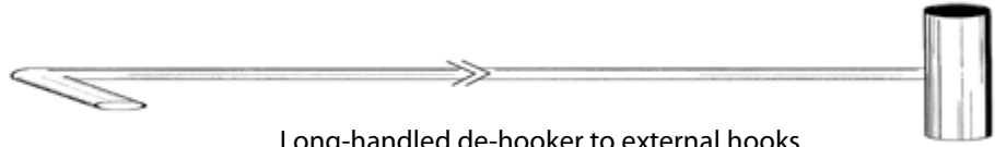
Long-handed de-hooker to external hooks
